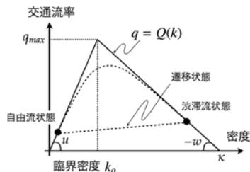
図-1 Fundamental Diagram
